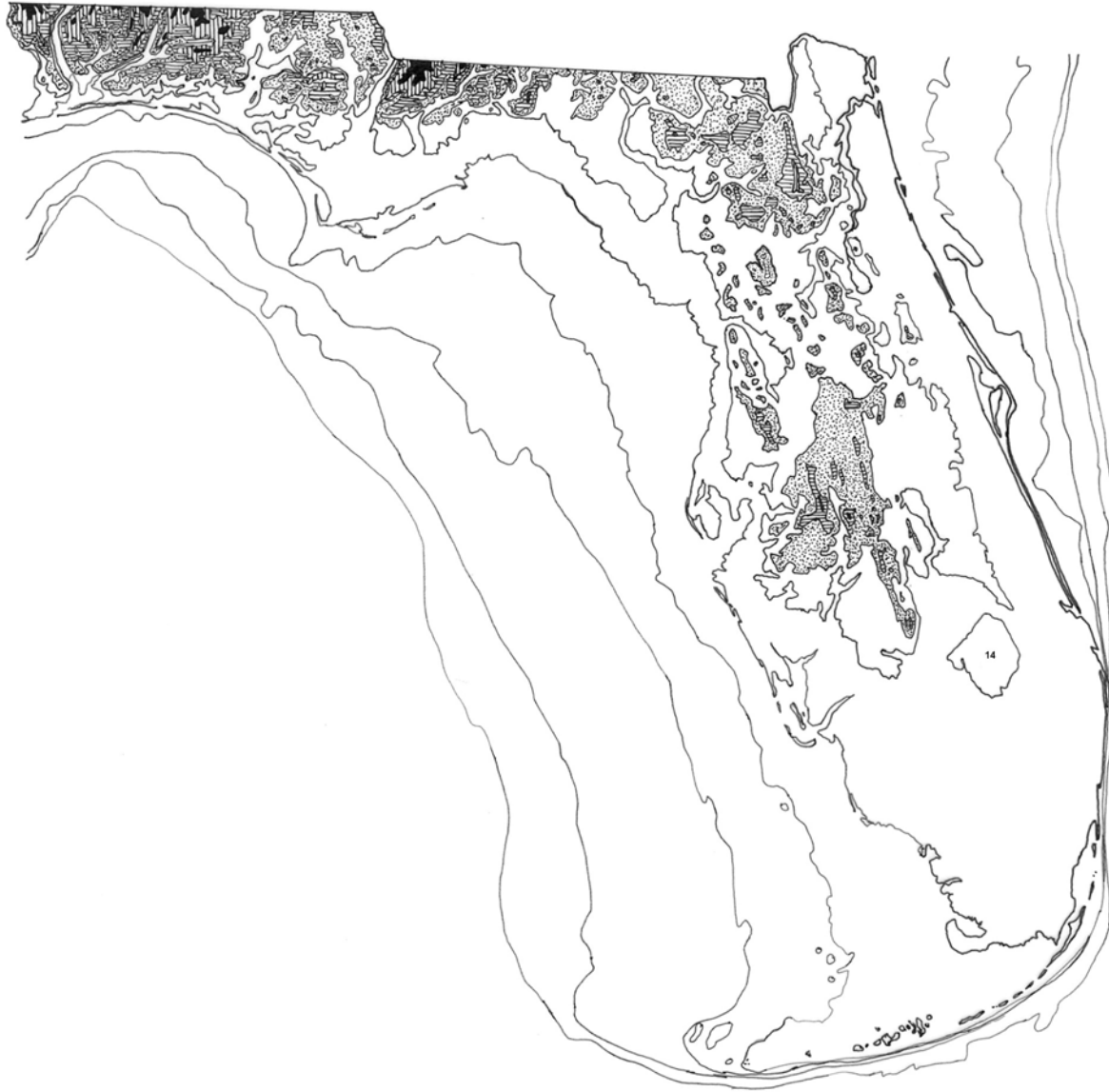
Fig. 11. Topography of Florida and offshore sea floor: 100 fathoms to 100 meters inland (intervals are ca. 25 m). Elevation of Lake Okeechobee is 14 ft (3 m) (after Fernald (1981), Atlas of Florida ).
